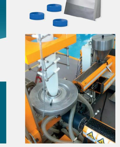
equipment is used in the project to obtain pellets by reactive extrusion from biodegradable material grades and reticulate agents. The chemical modification succeed on biodegradable materials with improved thermal properties and similar mechanical properties to the current commercial materials without affecting the shelf life of the dairy products.
